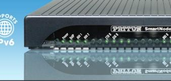
With up to 4 BRI ports and 8 simultaneous G.711 voice channels, the SN4130 is the best way to connect ISDN networks or ISDN terminal equipment to the world of voice over IP. With built-in security features such as HTTPS provisioning, Stateful Firewall and optional SIP-TLS<sup>\*\*</sup> it provides business-class Internet telephony for demanding ISDN users.
